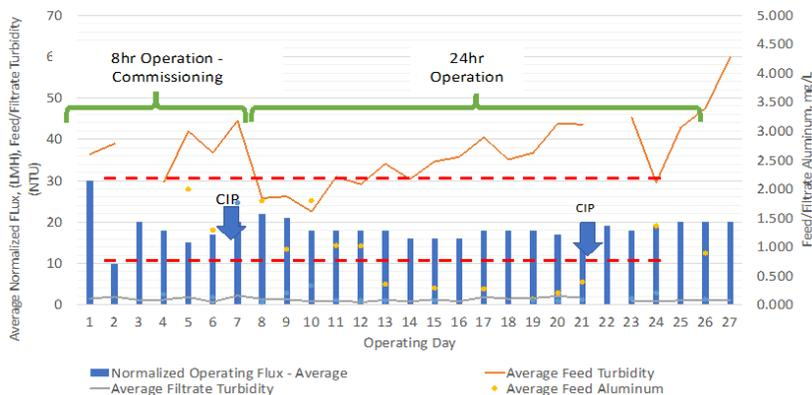
The pilot demonstrated 77% recovery with the single stage RO operation, yielding a treatment cost of \$0.65-0.75 /m<sup>3</sup>, 81% reduction in brine disposal volume, and generation of a solid waste which can be classified as a non-hazardous waste.
